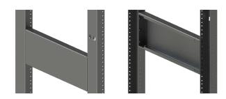
OPTIONAL: Connect Middle Depth Panel using provided #12-24 screws / cage nuts as needed.
